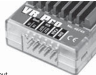
During working, the built-in tri-color monitor displays battery voltage: over 7.4V with green light, 7.4V to 7V with yellow light, lower than 7V with the red light. When the red light on, the user should stop using as soon as possible. The red light warning has memory function, it indicates that the battery has fault (low voltage, poor contact or system overload). Close the switch and re-open it can reset the memory.
